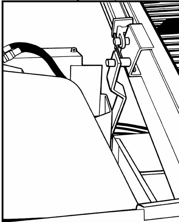
4. Extend the discharge conveyor main cylinder (this will lift the discharge conveyor from stored position to upright position).
