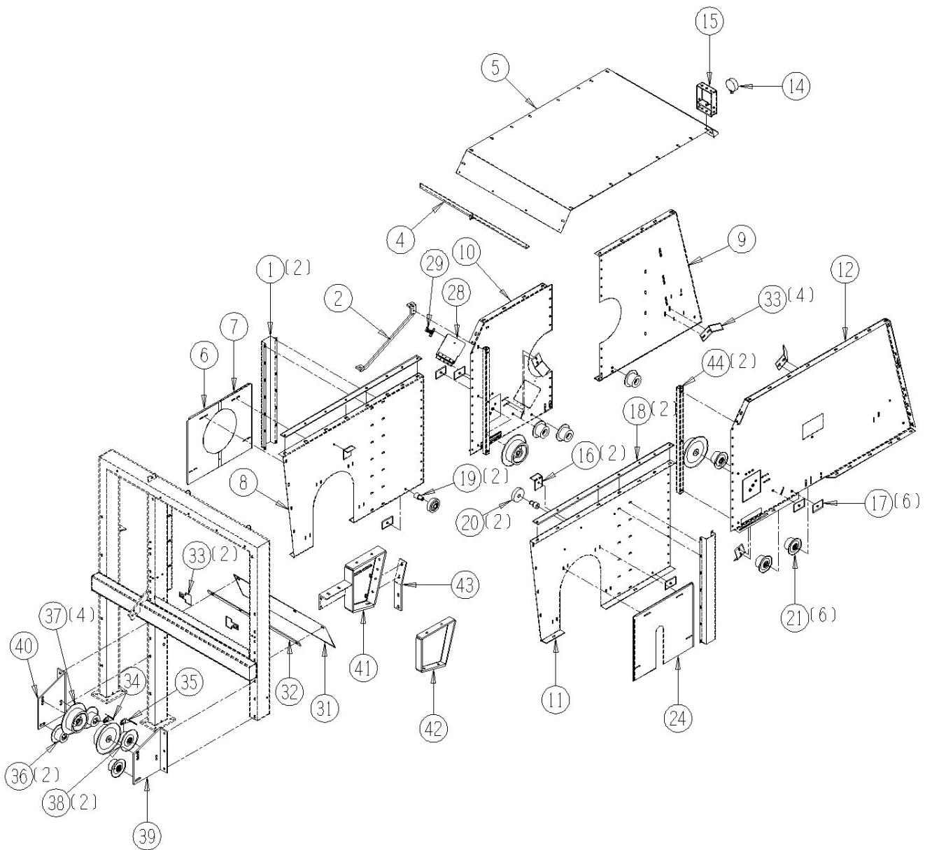
10010-04-51      Optional Shaker Chamber Box Shield Assembly
