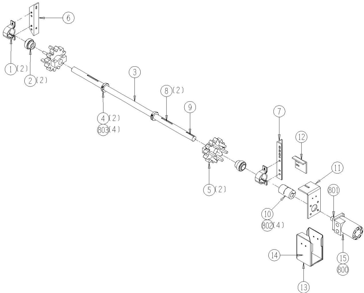
10010-08-07 Opt. Elevation Conveyor Bar Cleaner Assembly
