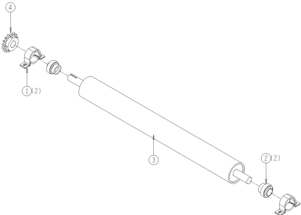
10010-03-11 Header Conveyor Vibrator Shaft Assembly
