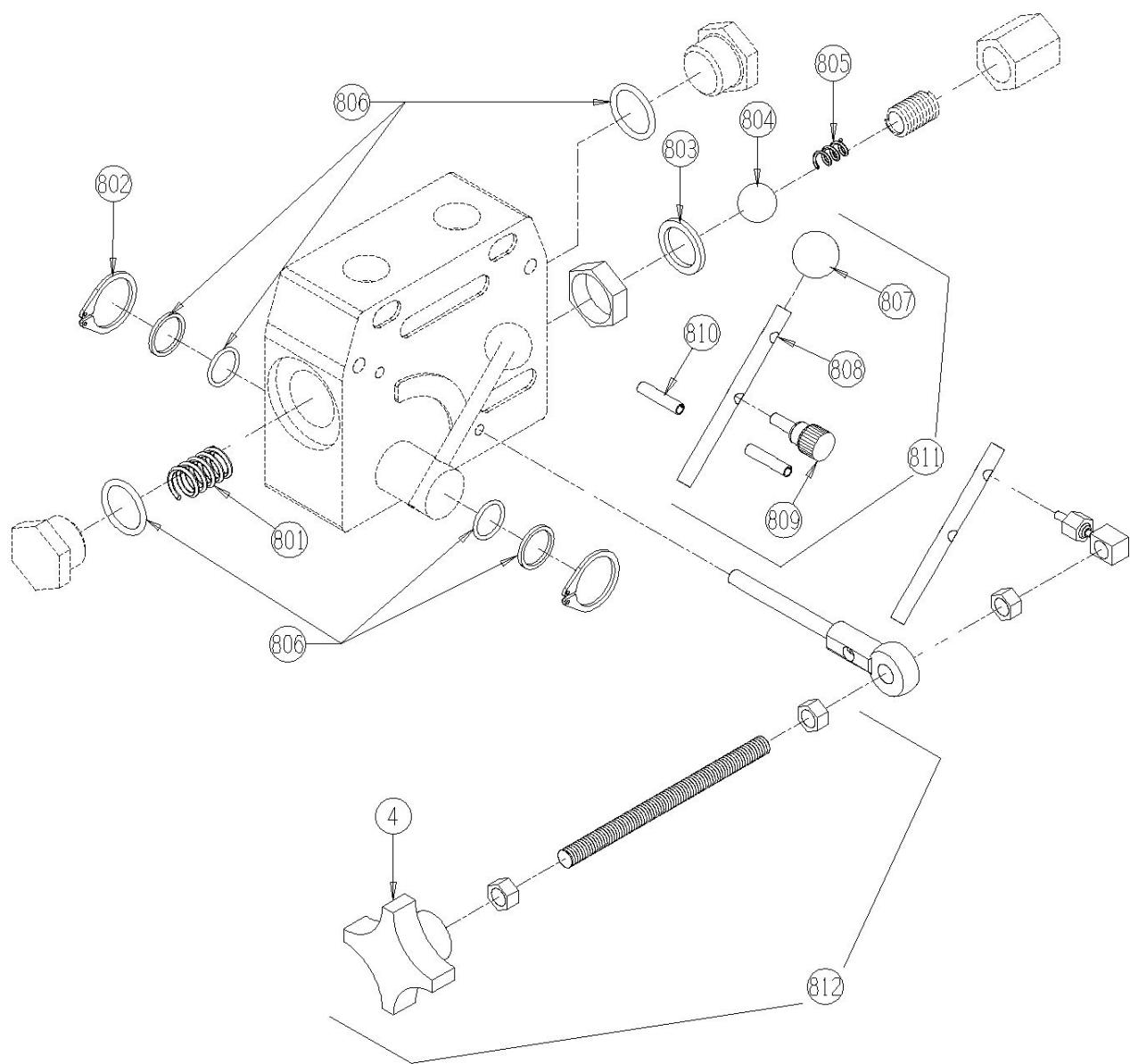
10010-80-05      Hydraulics, Relief Valve Parts Assembly
