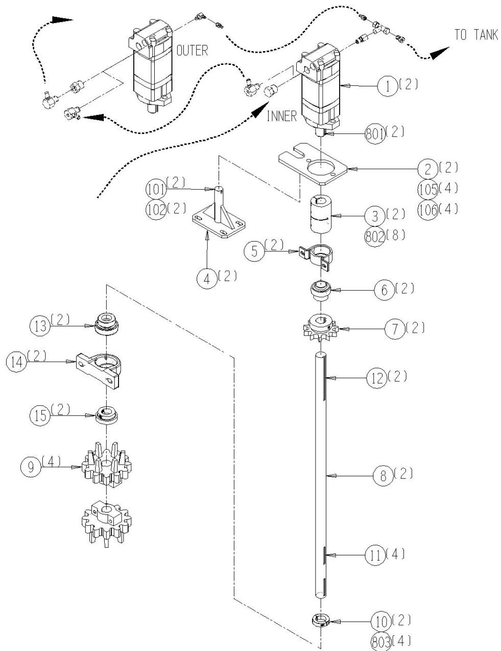
10010-02-03 Disk Header 34' Disk Shaft Assembly
