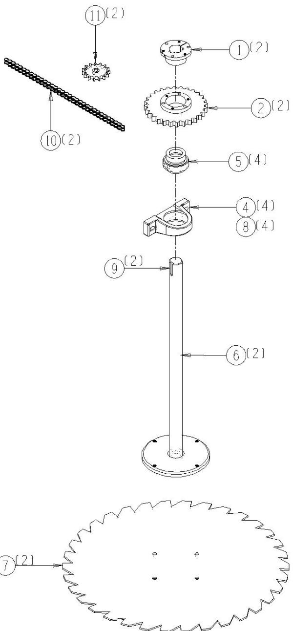
10010-02-04 Disk Header 36" Disk Shaft Assembly
