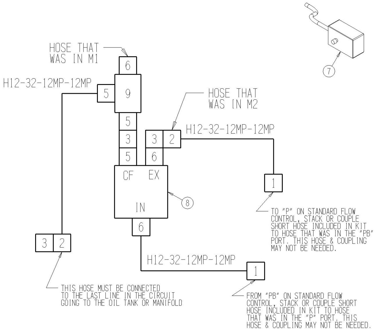
1109-15-21      Electronic Flow Control (3/4' Lines) Assembly
