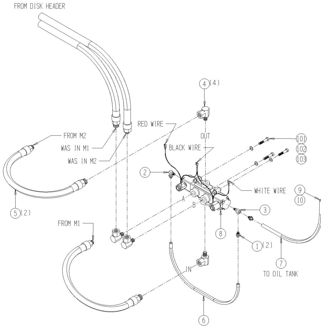
1109-15-20      Electronic Flow Cn (3/4' Lines w/Relief) Assembly
