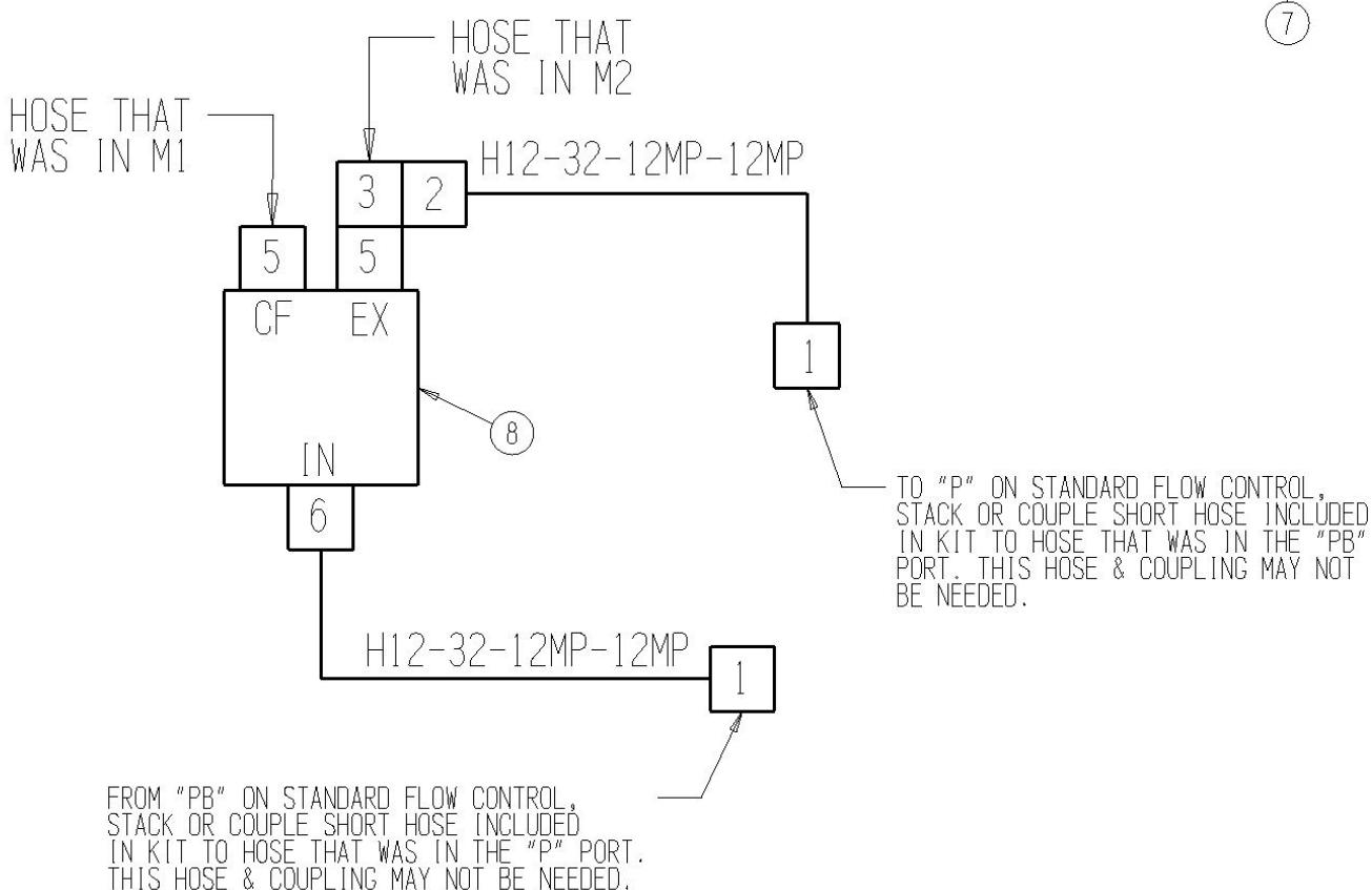
1109-15-22 Electronic Flow Control (5/8' Lines) Assembly
