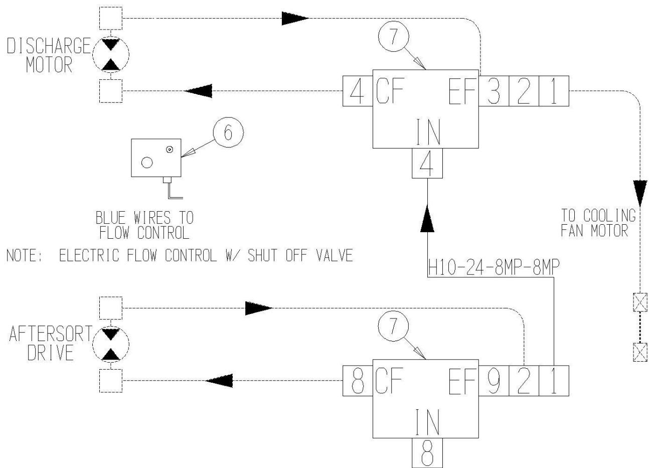
11010-15-07 Header Component Valve Section Assem.
