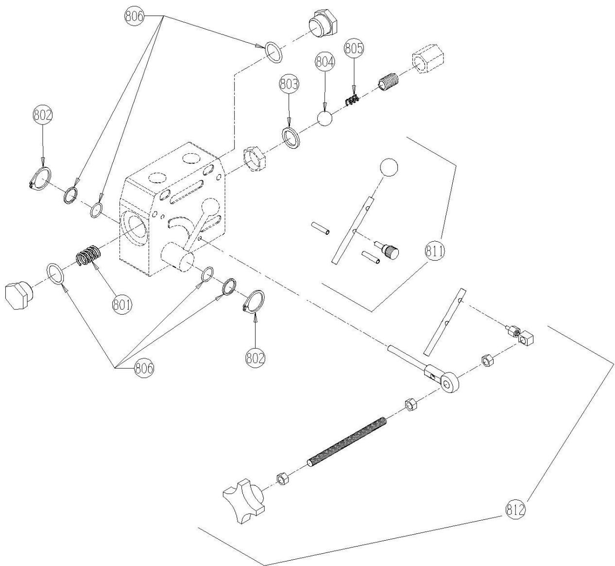
11010-15-24      Hydraulic Panel Component Mounting Assembly
